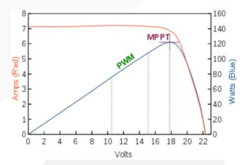
Image 1. Typical output curve solar panel
