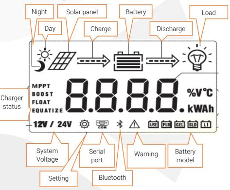
During start-up the 4 battery charging indicators will successively start to flash, and after the self-inspection the LCD-screen will be started and the battery voltage level will be displayed. This is a fixed voltage value chosen by the user or a voltage that is automatically recognised.
