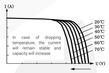
Voltage will decrease in case of an increase in temperature Image 2. Relation between solar panel output and temperature
