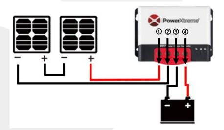
Image 8. Wiring diagram for the charge controller of several solar panels in series.
