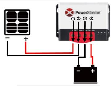
Image 2. Wiring diagram charge controller one solar panel
