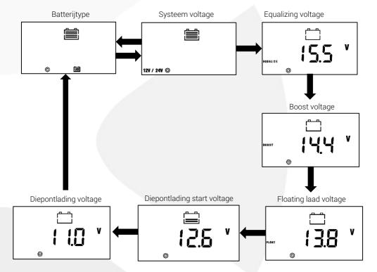
Once you are in the menu, press the Set button again to get to settings. Adjust the value with the up and down buttons. Then press the return button to close (without saving or setting parameter), or hold down the Set-button to save the settings and close.
