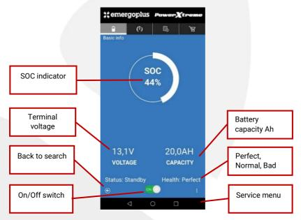
SOC means "State of Charge" or the state of charge of the battery. The voltage and capacity of the battery are listed below.
