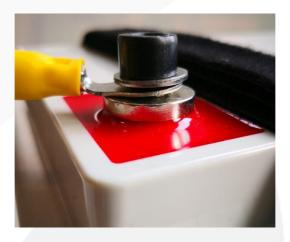
Figure 3. WRONG! Loose connection by using too long bolt
